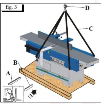
• Provide for a fork lift truck A with the respective load capacity, corresponding to machines weight;
