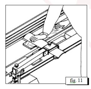
• The piece is pushed forward on the entry board by the palms of the hands, the hands passing one after another over theguard of the cutting shaft (fig. 11,12).
