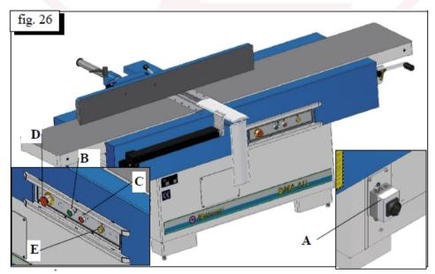
A - Main switch – serves for inclusion and switching off of an electric feed of the machine. There is an opportunity to stop a switch, having closed it on the lock, in position "0" with the purpose to avoid possible undesirable start-up of the machine. It is put in action by turning. Position "1": "is included". Position "0": "is switched off".
