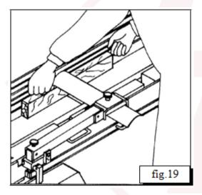
The piece is pushed forward by the palms of both hands, exactly as for details thick up to 65 mm (fig. 11, 12, 13).
