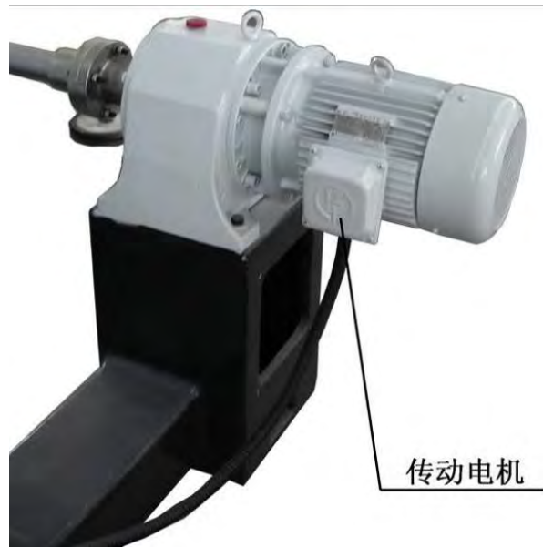
传动电机-motor for transmission system
